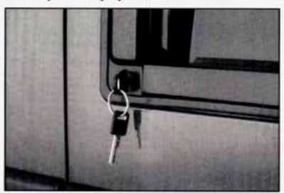
To release the hatch and unlock the doors from the outside of the vehicle, put the key in the lock and turn clockwise. Then, pull up on the hatch and open the right rear door first. Grasp the handle and pull the door open.
